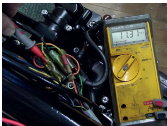
Ignition ON, coil reading 11.31 volts
